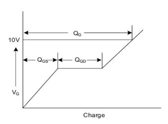
Fig. 3.2 Gate Charge Waveform
