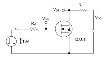
Fig. 2.1 Switching Test Circuit
