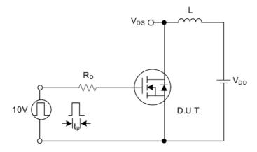
Fig. 4.1 Unclamped Inductive Switching Test Circuit
