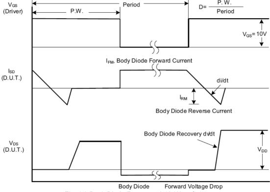
Fig. 1.2 Peak Diode Recovery dv/dt Waveforms
