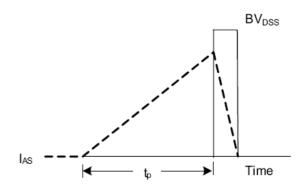
Fig. 4.2 Unclamped Inductive Switching Waveforms
