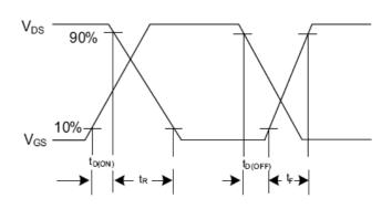
Fig. 2.2 Switching Waveforms
